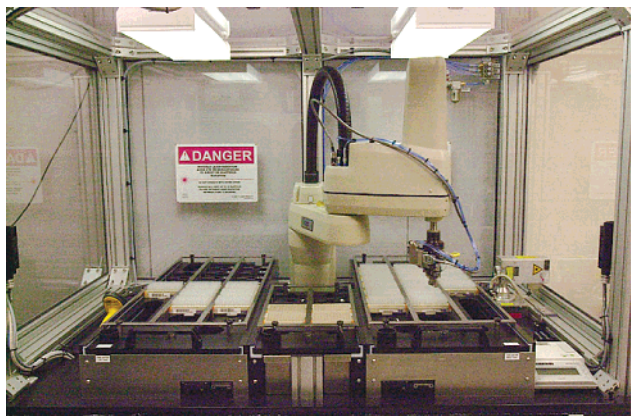
Figure 2. Custom GNF tube labeling, sorting, and weighing robot.
